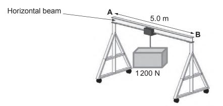
When the gantry crane supports a load of 1200N at its centre, a force of 700N is exerted on each pillar. Calculate the weight of the horizontal beam. [2]
