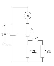
In the circuit shown, with the **switch open**, the ammeter reads 0.5A. Show that  $R = 6\Omega$ . [2] (i)
